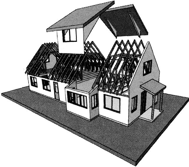
Fig. 2. 1-1/2 story prototype as built: Open panels with exterior finishes and windows installed at factory; panelized interior partitions; attic trusses; double girder trusses supporting panelized dormers and central floor cassette.
